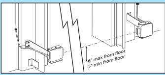
FIG. 5-4 Check Safe-T-Beam® alignment.
